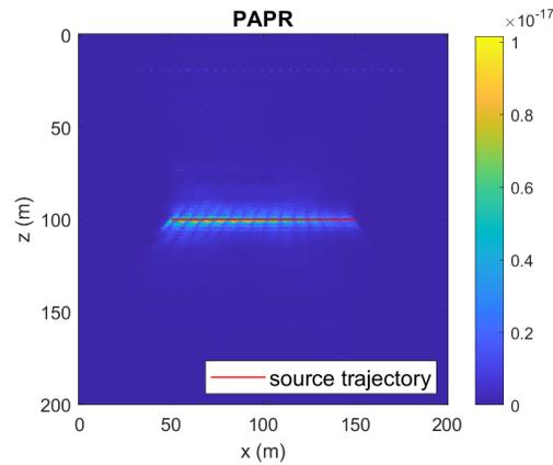
**Figure 6.** Snapshot of the resulting wavefield for a homogeneous model at the final time instant with the linear moving source acquired using the PAPR coefficient.
