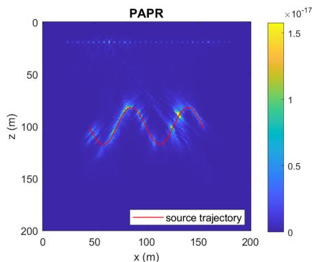
**Figure 8.** Snapshot of the resulting wavefield for a homogeneous model at the final time instant with the sinusoidal moving source acquired using the PAPR coefficient.
