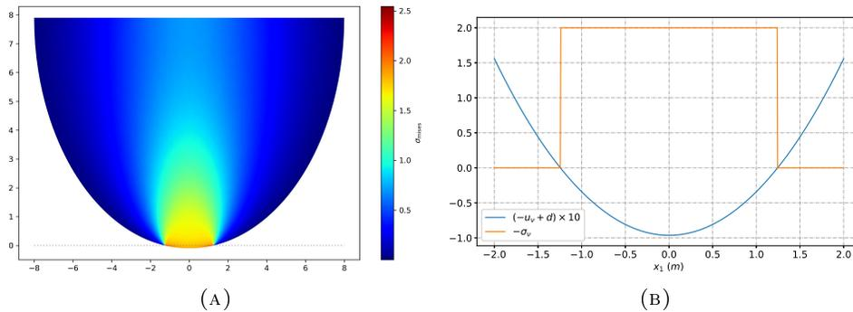
Рис. 6. Deformed configuration and von Mises stress (A), normal stress, displacements for  $\xi = 2$  (B) on  $\Gamma_c$ .
