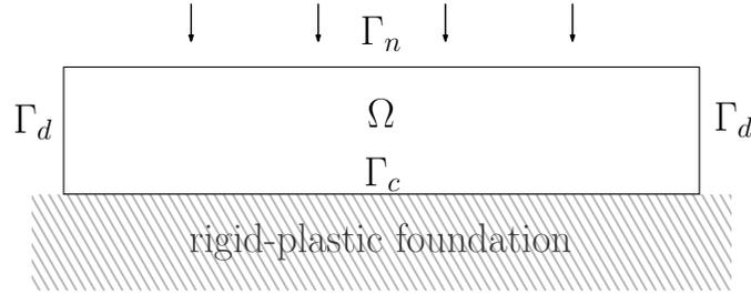
Рис. 1. Contact with rigid-plastic foundation.
