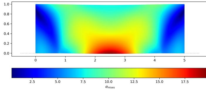
Рис. 4. Deformation and Von mises stress with  $\xi = 16$ .
